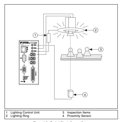
Figure 4-9. Typical Single-Camera Setup
